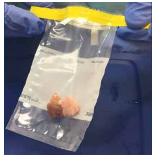
Figure 17. Whirl-Pak® type bags are sealable, leak-resistant, and can be used for storing and transporting samples.
