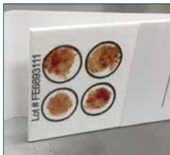
Figure 7. Completely dry the sample on the card by placing the card on its side.
