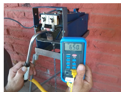
Pyrometer indicating proper blade temperature of 650°C.
