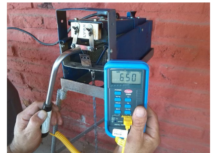
Pyrometer indicating proper blade temperature of 650°C.
