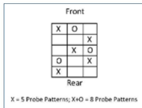
Figure 5. An example of a 5- and 8-probe sampling pattern (43).
