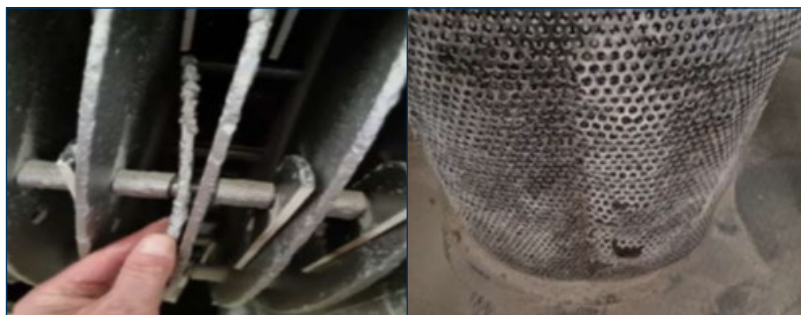
Figure 2. Excessively worn beaters (left) and punctured screen (right).
