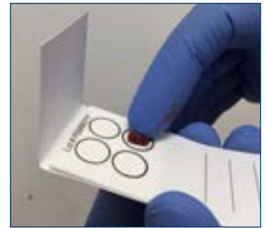
Figure 6. Lightly press the tissue onto the FTA card and remove excess tissue.
